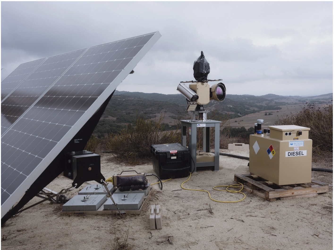
Anduril's sentry towers run on solar panels, making them easier and cheaper to install.
